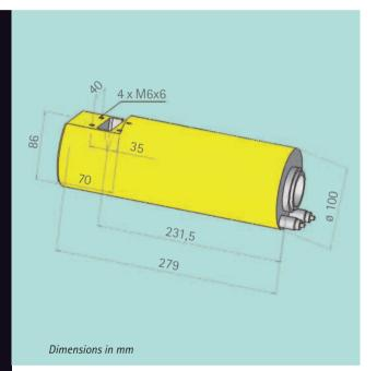
YXLON end grounded metal-ceramic X-ray tube with a 60° fan beam is especially suited for inspection tasks, which need a wide X-ray beam.
