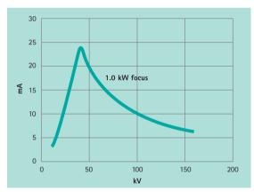
**Loading data:** Shown are the max. permissible anode currents. Within the X-ray system these anode currents may be limited by power suppliers or generators.
