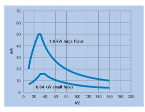
**Loading data:** shown are the max. permissible anode currents. Within the X-ray system these anode currents may be limited by power suppliers or generators.
