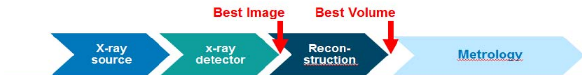
Figure 7: The process of producing reliable metrology results.
